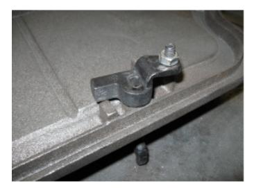
5. Use the provided spreader tool and a ball peen hammer to spread the "fingers" of the knob outward to secure the latch. Spread them wide enough to hold the latch firmly Do not over tighten. There should be some play in the knob.
