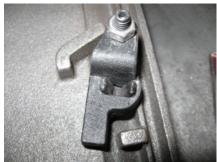
6. Place the door back on the door frame. Tap the hinge pins down all the way.
